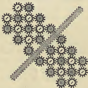
FIG. 39.—A provisional representation of a current surrounded by dielectric medium, either propelling or being propelled. Section through the wire.
